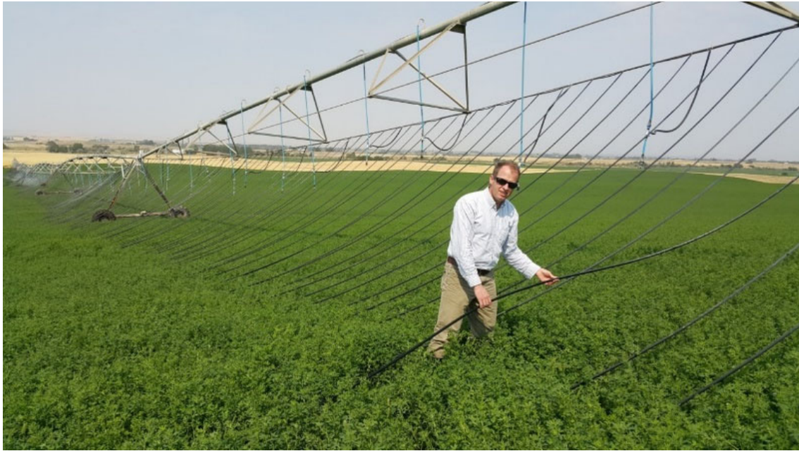
Figure 7. Using of MDI on alfalfa in Oregon in 2017. MDI does not wet a significant part of plant canopy, which makes it easy to walk through and maintain the field as needed.
