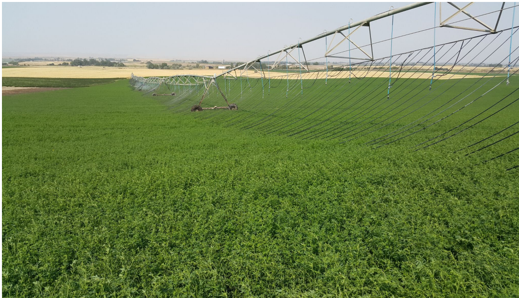
Figure 12. Alfalfa irrigation using a center pivot with a mobile drip irrigation (MDI) system in Umapine, Oregon. The MDI systems are extremely efficient and apply water slowly to permit greater infiltration depths per pass. (photo by Behnaz Molaei).
