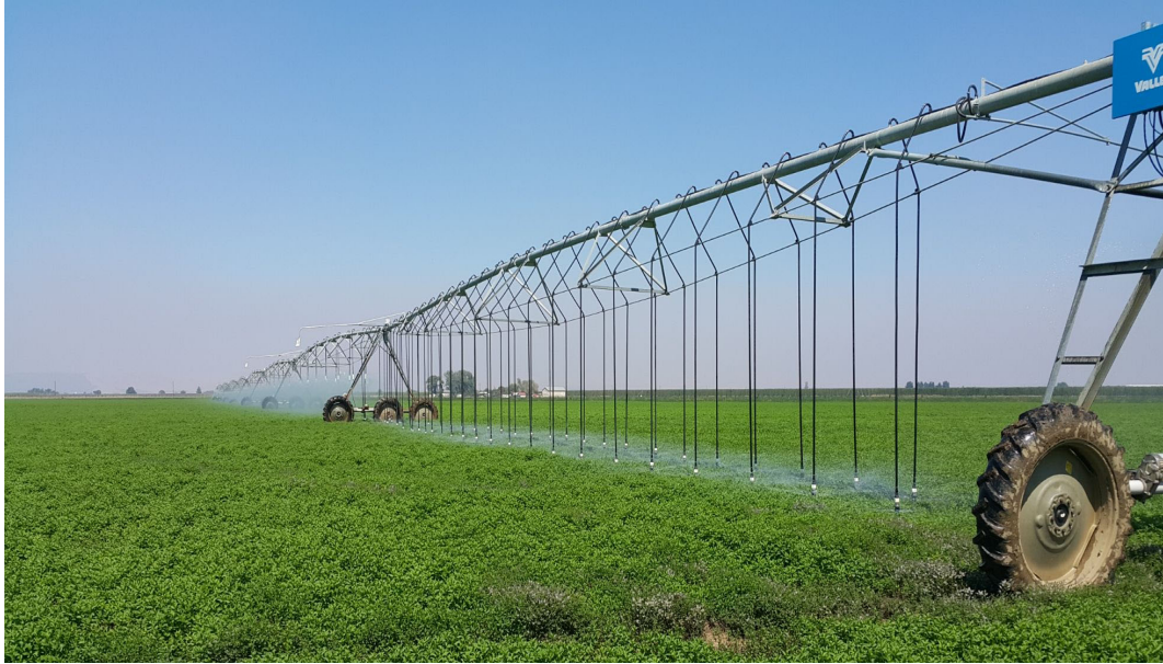
Figure 11. Center pivot irrigation with low elevation spray application (LESA) and with mid elevation spray application sprinklers (MESA) operating in the background irrigating the spearmint field in Toppenish, Washington (photo by Behnaz Molaei).
