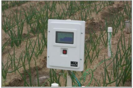
Figure 1 shows the AM 400 developed by the M. K. Hansen Company mounted in the indoor/outdoor enclosure with a see-through window for the DGI display. Up to six watermark sensors can be logged by a single AM 400 along with two temperature sensors (thermistors) used to measure soil temperature and to correct the soil moisture data. Soil moisture and temperature are logged three times per day, once every eight hours. By initially
