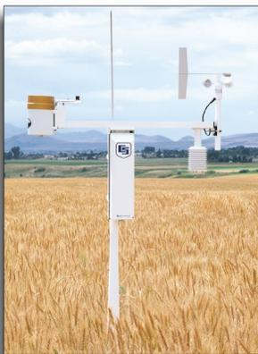
*Irrigation needs can be estimated using the ET106 Evapotranspiration Station.*
