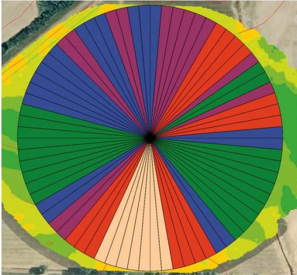
Figure 1. Variable Speed Irrigation. The pivot varies travel speed to apply variable amounts of water to defined zones within the field. Colors indicate areas with different amounts of water applied. Image used by permission from pivotirrigation.com.au.
