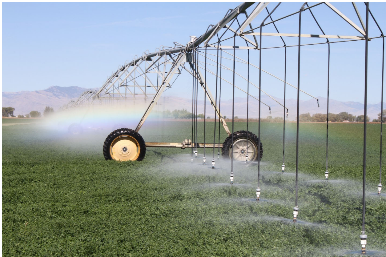
Figure 1. Mid Elevation and Low Elevation Spray Application (MESA and LESA). The difference in wind drift between the two systems is clearly visible. Losses from the droplets to evaporation are not visible (water vapor is transparent).
