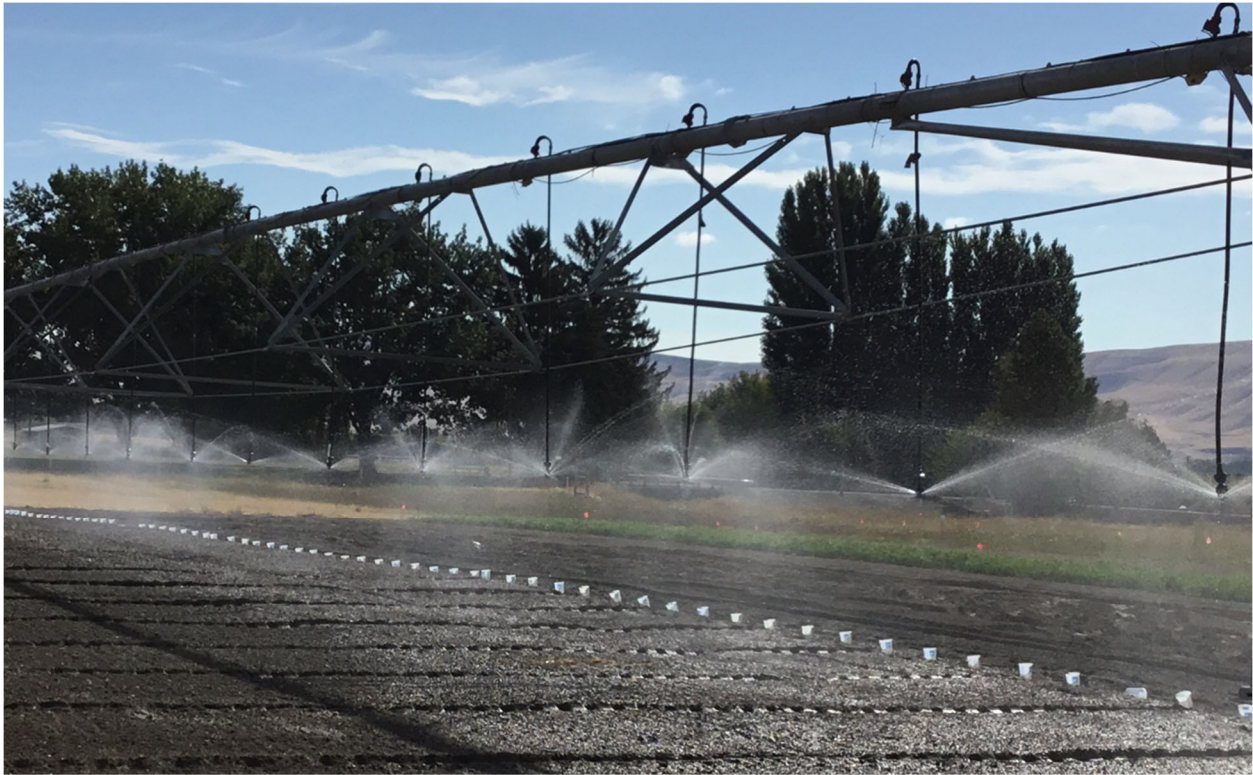
Figure 11. Catch can method to estimate the sprinkler water losses.
