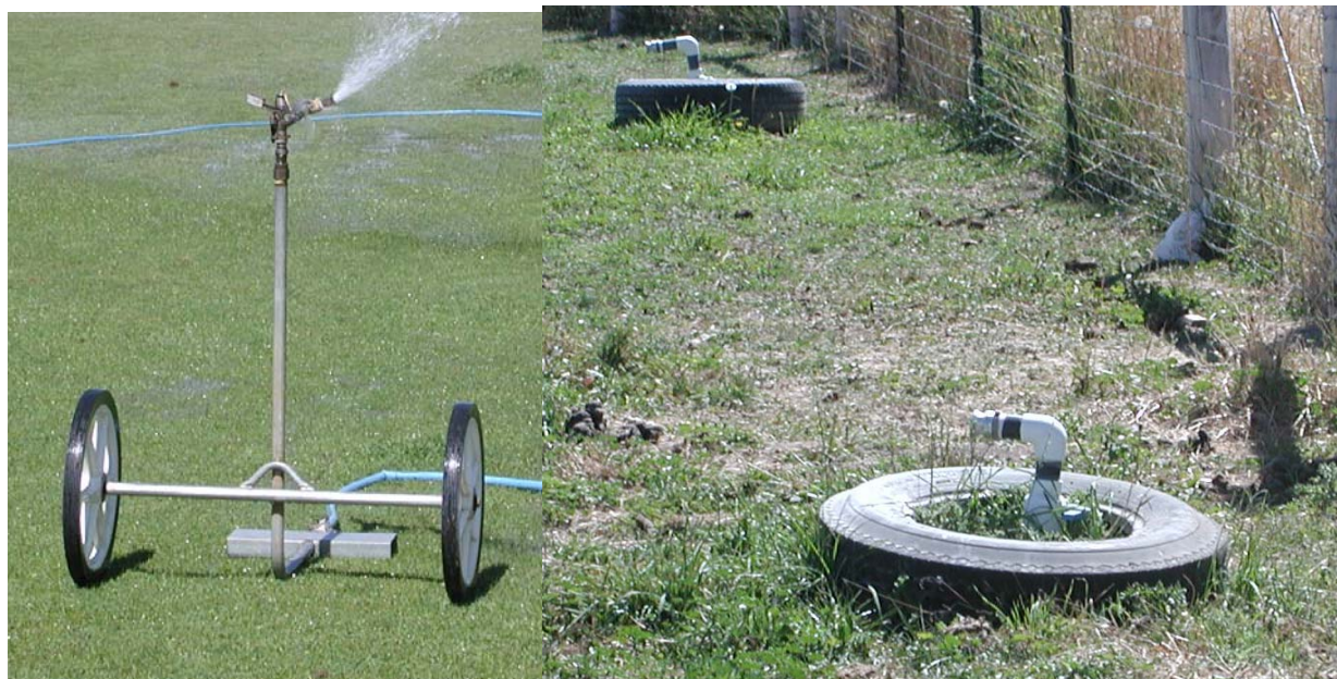
Figure 4. (left) Portable “big gun” sprinkler for pasture use (available from Farmore Irrigation, Jerome); (right) water supply risers in pasture. Risers outside the fence or in the fence line are less likely to be damaged by livestock or machinery traffic. Minimum hose size for proper operation is 1.5 inch. Note the poor pattern from this sprinkler, which is supplied with a \frac{3}{4} inch diameter garden hose.
