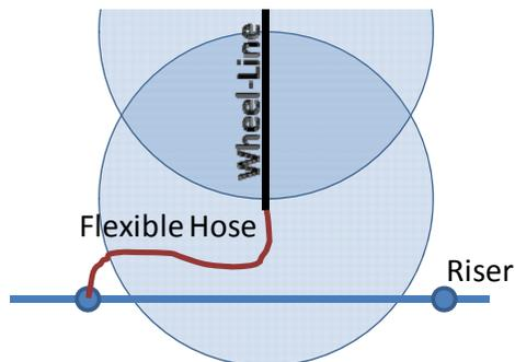
Figure 5. Using an offset on every-other irrigation cycle can significantly improve application uniformity.
