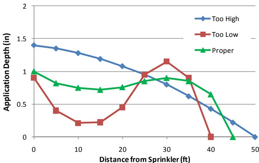
Figure 6. Application depths (patterns) with respect to distance from sprinkler head for pressure settings that are too high, too low, and properly adjusted.
