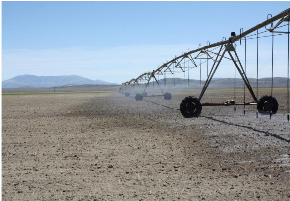
Figure 23. Due to its smaller wetted diameter, LESA allows less time for water to infiltrate into the soil. Therefore LEPA or LESA may not be suitable to tight soils or steep slopes where infiltration and runoff can be an issue.
