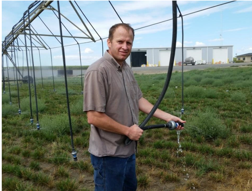
Figure 19. Sprinkler maintenance is much easier and can be done while the system is running while simply wearing irrigation boots without getting overly wet.
