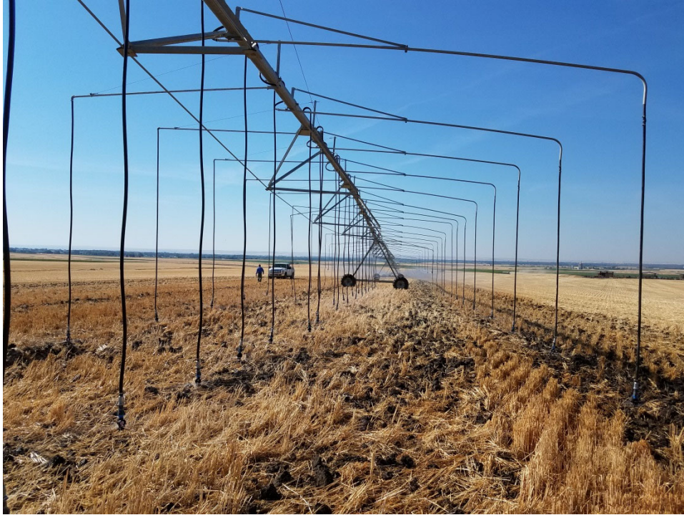
Figure 8. LESA system using boombacks to spread the water out and increase infiltration on a wheat field near Milton Freewater, Oregon.
