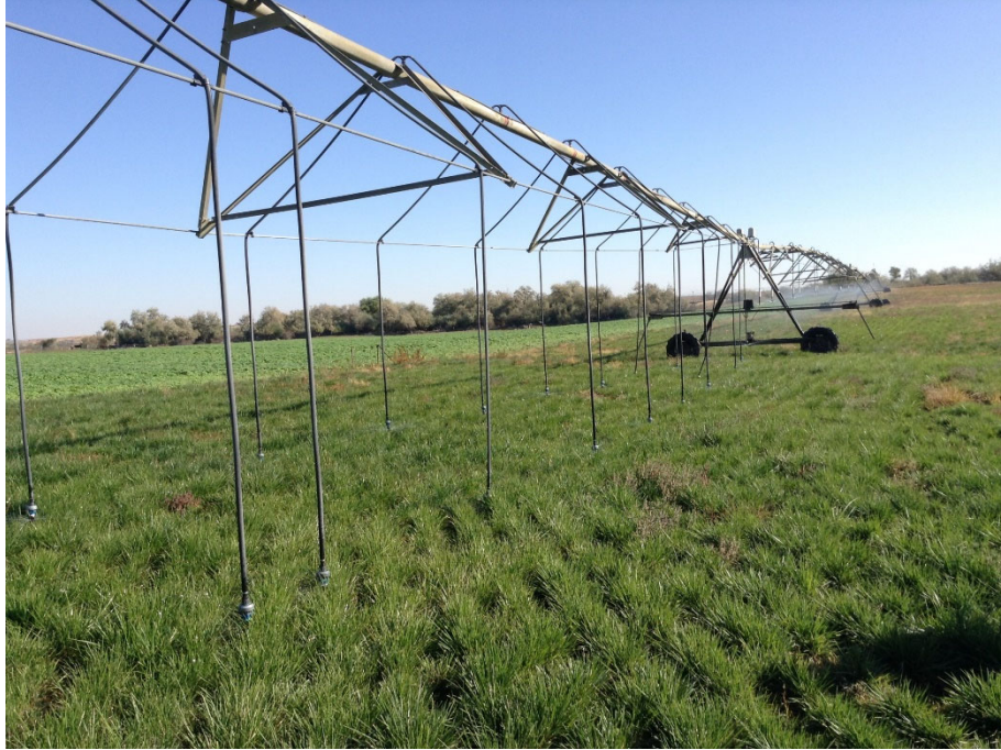
Figure 11. Double goosenecks and truss-rod hose clamps to position the sprinkler correctly are used to increase the number of sprinkler drops (decrease the drop spacing) without requiring additional outlets in the pivot pipe.
