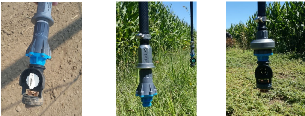
Figure 15: Examples of the sprinklers with the Nelson D3030 sprinkler bodies that drug through the corn. Possibly because of the sprinkler design, we found some losses of sprinkler spray plates,
