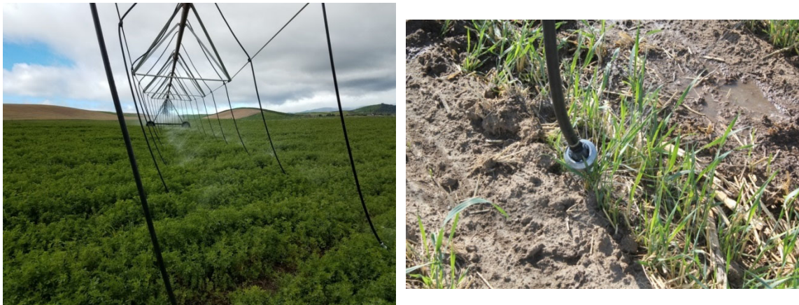
Figure 13. In some instances, sprinkler heads bumped along the ground due to deepening wheel tracks or undulating topography. Although no damage was noted to either the crop or the sprinklers, it bothered the farmer so we increased the height of the sprinklers (shortened the hose) a few inches in the LESA section
