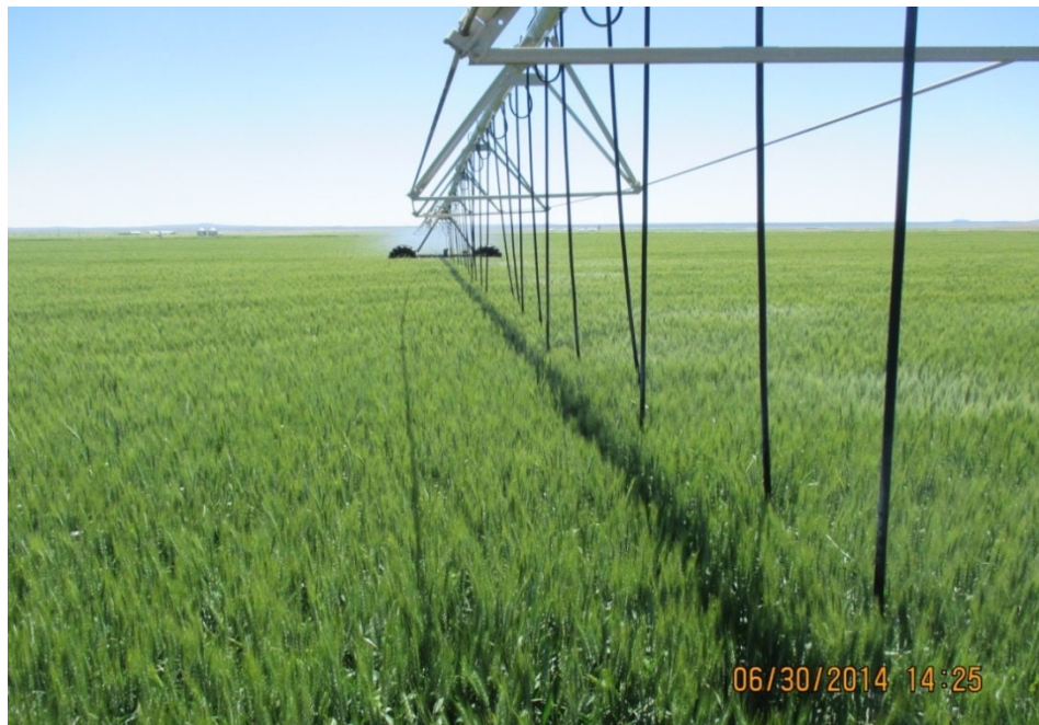
Figure 7. LESA operating in wheat with the sprinkler heads below the top of the canopy.
