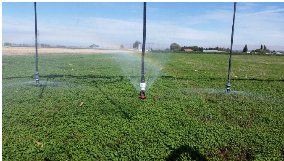
Figure 24. Chemigation plates can be used to spray water upwards to improve canopy wetting for chemigation.
