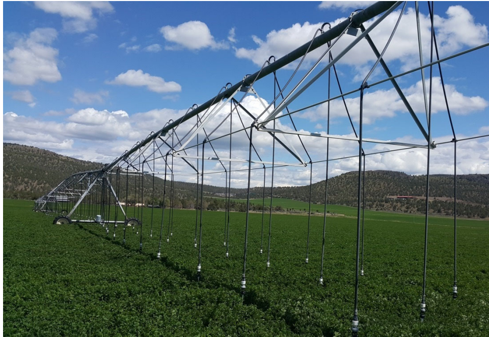
Figure 6: LEPA on alfalfa in Oregon where triple sprinkler drop goosenecks are used to increase the number of sprinkler drops (decrease the drop spacing) without requiring additional outlets in the pivot pipe or truss-rod hose clamps to position the hose correctly.
