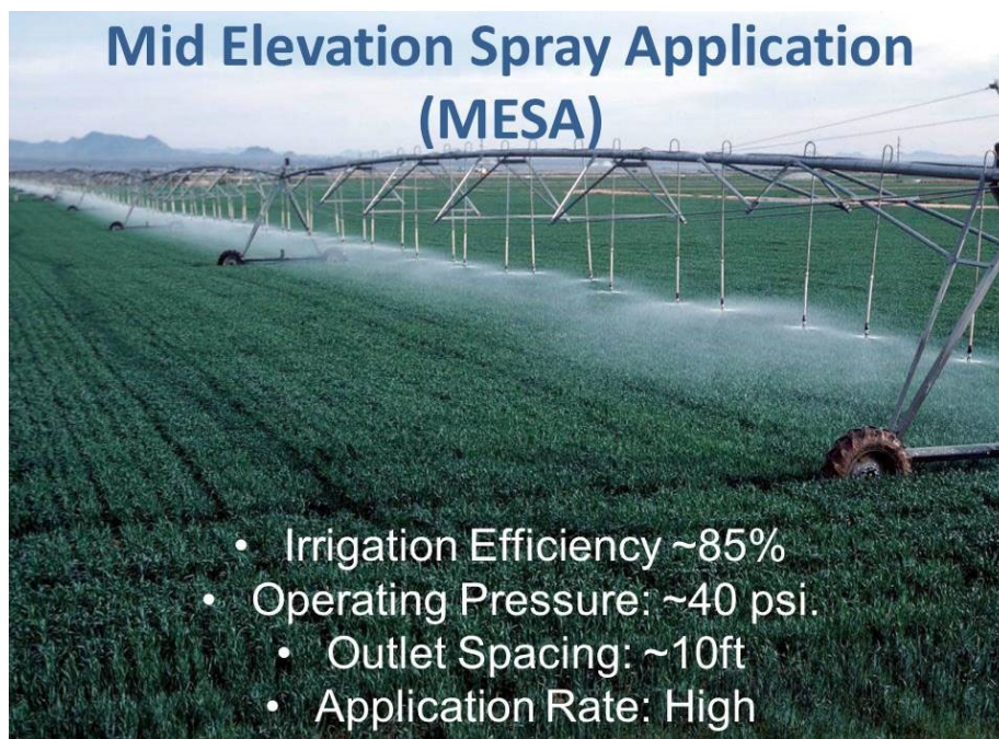
Figure 2. Currently most center pivots use mid elevation spray application (MESA). These sprinklers typically use 15-20 psi pressure regulators and thus need about 35-40 psi at the pivot point to operate properly. They are spaced about 10 ft apart, and the irrigation application efficiency is typically about 85% as measured with catch can tests without canopy. The smaller wetted radius does not allow as much time for the water to infiltrate into the soil as the pivot passes.
