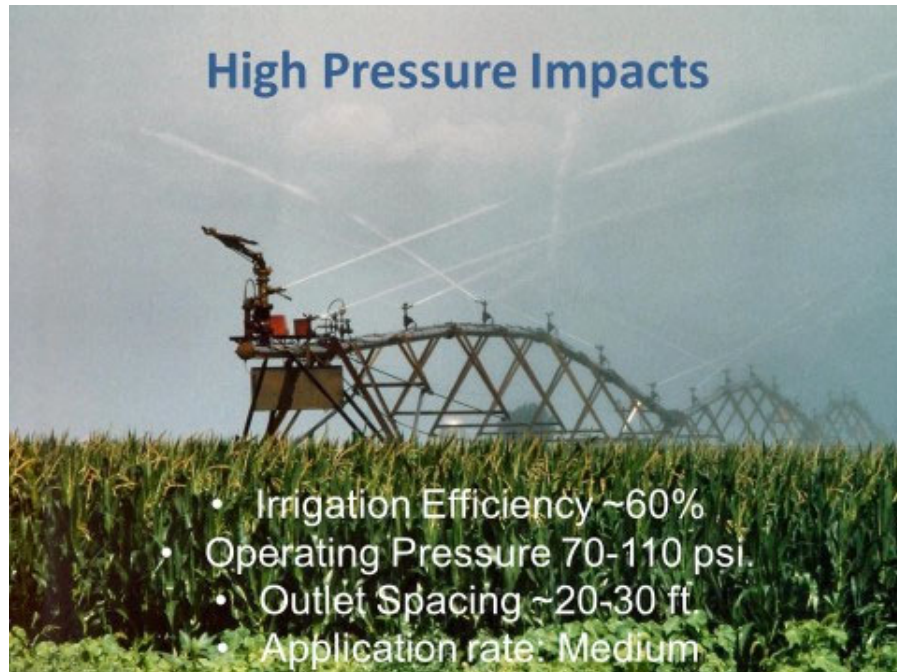
Figure 1. When center pivots were first introduced, they used high pressure impact sprinklers located on top of the pipe. These sprinklers needed 70-110 psi at the pivot point to operate properly, were spaced 20-30 ft apart, and the irrigation application efficiency was about 60% as measured by catch can tests without canopy. However, due to the large wetted radius, there is more time for the water to infiltrate into the soil as the pivot rolls past.
