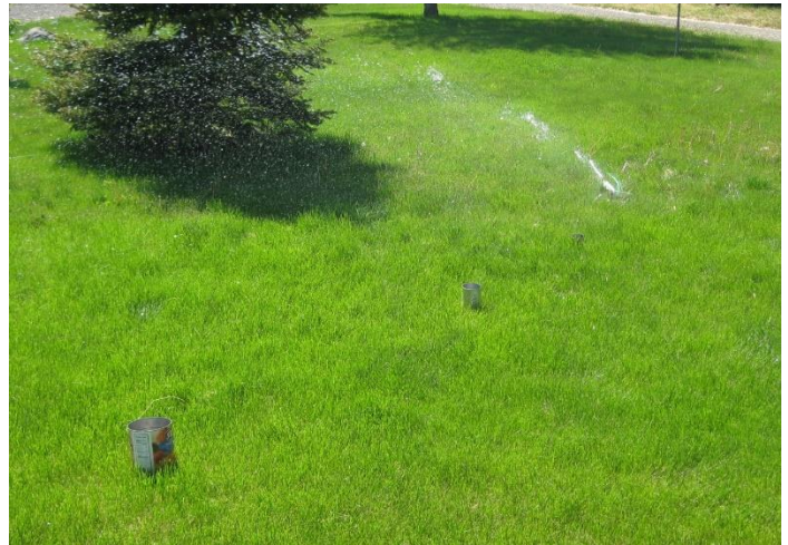
Figure 2. Cans laid out to measure water application depth. Photo: R.T. Peters.
