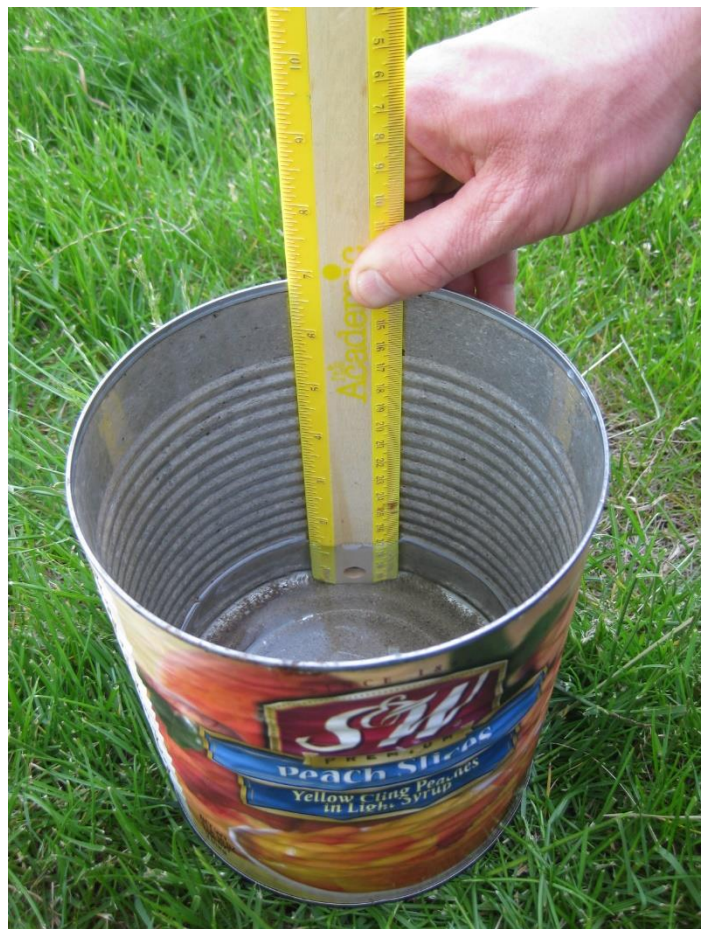
Figure 3. Measuring application depth. Photo: R.T. Peters.
